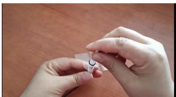
Figure 8. Securing and adjusting the membrane
