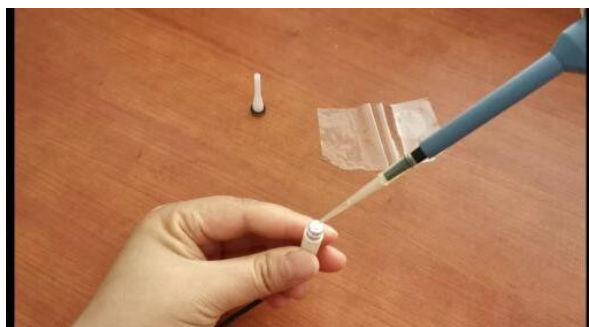
Figure 6. Applying electrolyte and positioning the membrane
