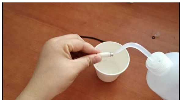
Figure 5. Cleaning the oxygen electrode
