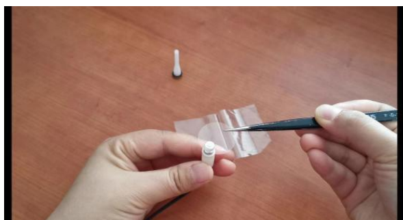
Figure 7. Installing the O-ring with the installation tool
