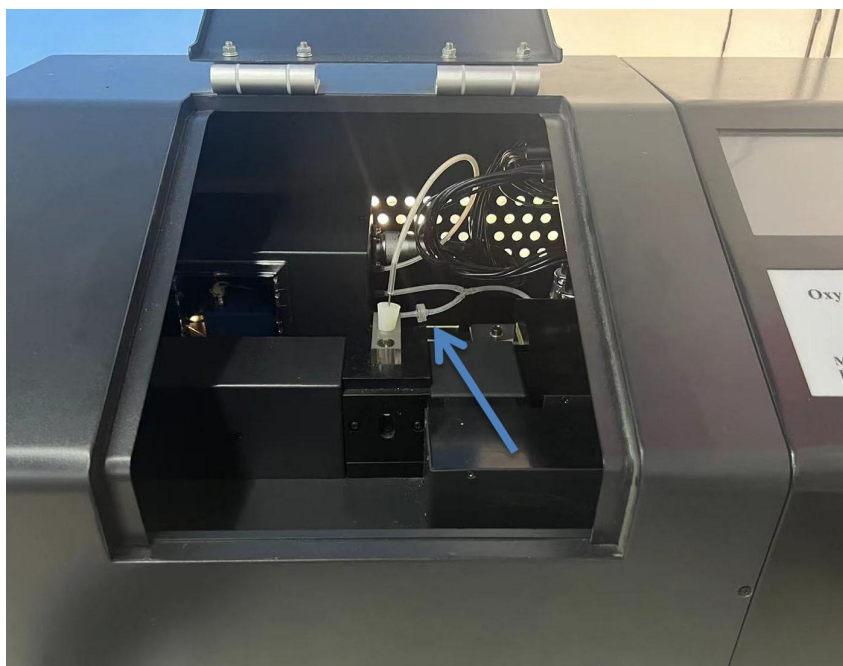
Figure 22. Sample-chamber area and gas-path components
